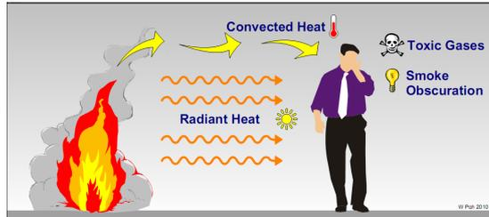
Figure 1 Exposure in Building Fire
